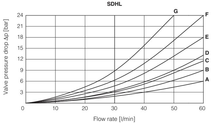
**10 OPERATING LIMITS** based on mineral oil ISO VG 46 at 50°C
