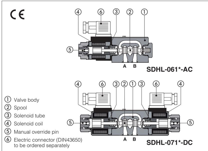
Spool type, two or three position direct operated valves size 06 in compact execution with reduced solenoids dimensions, ideal for applications in mini power packs, mobile and agricultural machines.
